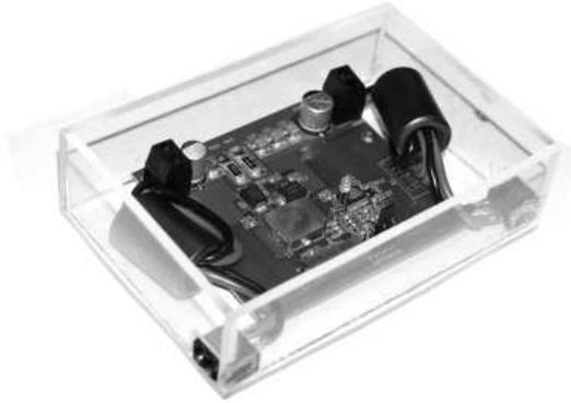
Figure 4: ELV “USW-525” universal voltage regulator in a case
