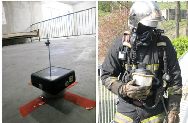
Figure 1: A first generation RELATE sensor node placement on the floor of the training facility and a firefighter equipped with several sensor nodes
